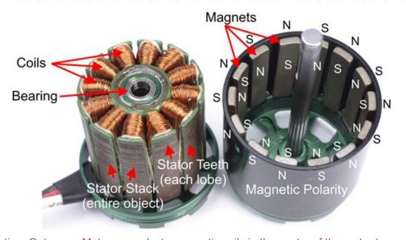
Caption: Outrunner Motors use electromagnetic coils in the center of the motor to drive permanent magnets attached to the rotating exterior can of the motor. This design yields a larger rotor diameter and can generate more torque than a similarly sized inrunner.
