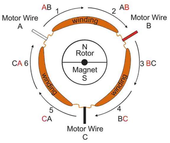
CAPTION: A precise sequence of power application and reversal is required to turn the shaft one full revolution. The three winding coils are each energized in 2 opposing ways using the three motor input leads, A, B & C. The combinations are color coded red for + and black for --. This drawing represents a two pole motor with each phase having only a single coil
