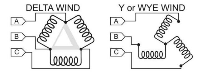
Without any outside influence (like a moving magnetic field) these motor winding circuits are dead shorts, which is exactly what the ESC has to deal with during startup or under heavy load.
