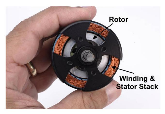
This Neumotors ORK uses a larger-than-normal rotor diameter and a high pole count to generate more torque at the shaft than a traditional inrunner motor. Motors with higher torque can often drive props without using a gearbox.
