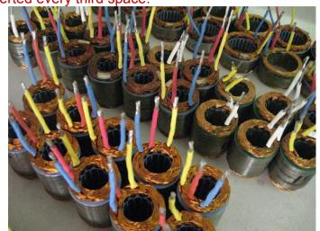
Caption: Wound stator stacks await assembly at NeuMotors. One stator size can have many different turns to make motors of different KVs.
