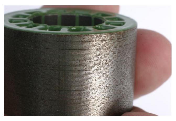
Caption: A stator stack is made of hundreds of rings of special steel which focus the magnetic fields generated by the copper wire that is wrapped around the "teeth" in the stator. More layers of thinner steel generally leads to a more efficient motor -- less heat for a given power output.
