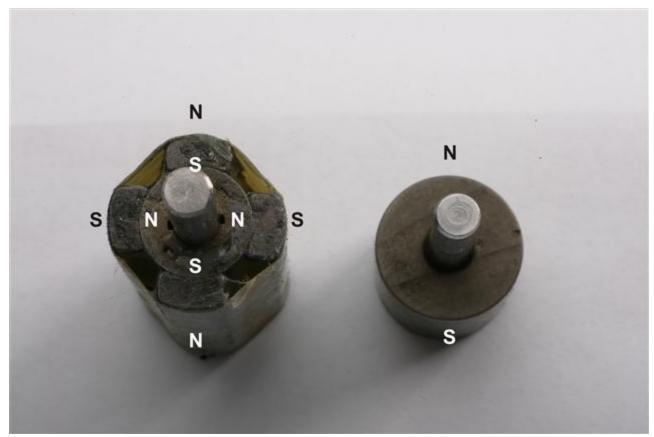
Inrunner motors generally have the permanent magnets bonded to the shaft, such as in the four pole rotor on the left. Two pole rotors (right) have the magnet surrounding the shaft. The integrity of these attachments determines the max RPMs of a motor. Some motors use a Kevlar (see rotor on the left) or carbon wrap to increase the strength of the attachment to the rotor.
