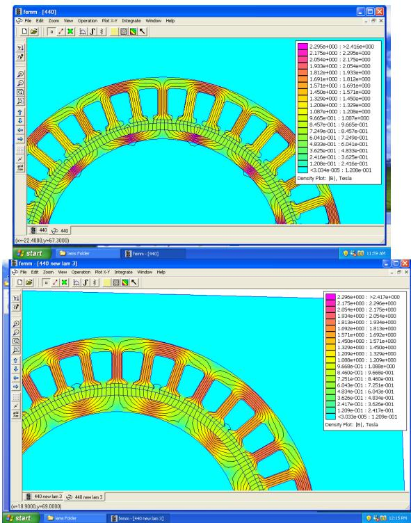
The screen on the bottom shows how changes to the shape of the tips of the stator teeth and increased "back iron" allowed the stator to perform at much higher power levels before reaching magnetic saturation and suffering the corresponding loss of efficiency as shown in the magenta portions of the top image. Tweaks like this can make a huge difference in performance characteristics.
