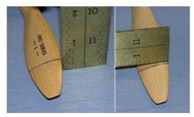
Measuring the pitch of a propeller is easily done on a flat surface with an accurate ruler.
