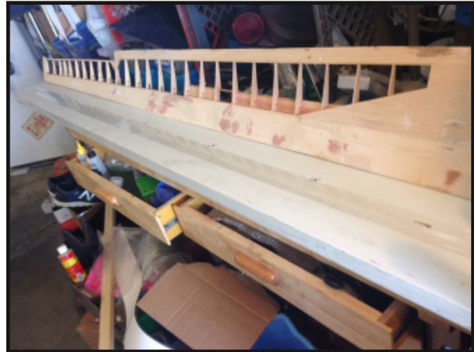
a) Lay-stretch 2 inch clear packing tape the length of the wing, sticky side up
