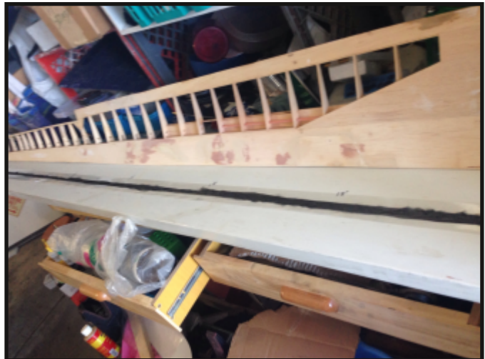
b) Stretch and lay carbon fiber onto the sticky side of the tape. Use a wide piece of balsa to spread, even out and flatten carbon fiber roving onto tape.
