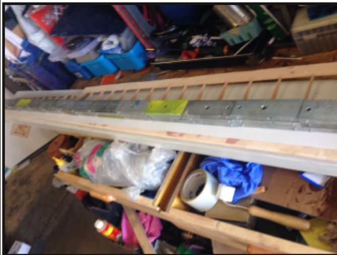
d) Apply uncured carbon fiber tape to the spar. Use a flat plastic blind with weights over the tape to achieve a smooth finish. When the epoxy is cured, peel the packing tape off, achieving a smooth finish.
