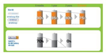
After a storage time of 3 years a eneloop battery still retains 75% of its inital capacity whereas a normal NiMH battery has no capacity left after 2 years. Some NiMH batteries have an even worse rate of self-discharge. A loss of 1% of its initial charge per day is not uncommon.
