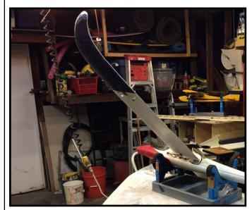
The ESCs are attached to the fuselage under the wing. No room for them under the canopy. To achieve the correct CG a large 3S-2200maH battery is pushed all the way forward in the nose. Flight times with that battery and modest power are about 25 minutes.
