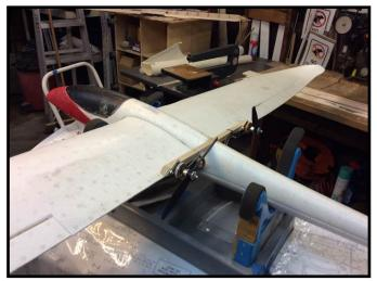
A close up of the twin pushers on a boom. A fair amount of down thrust, plus elevator mixed to the throttle, is needed to get a good glide and still keep the damn thing from looping under power
