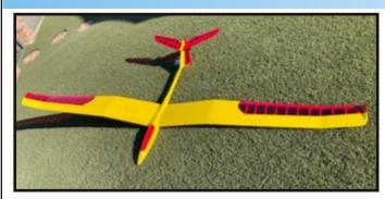
"I made some changes to the design. The original wingspan was 130 inches. I reduced it to 100 inches, for easier slope landing. (Bob uses Staples to print the PDF files to the size he wants. In this case, they printed the plans at 73%.)
