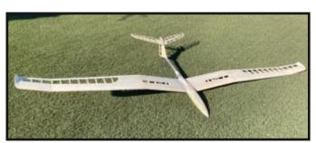
the wings. Also, the spoiler blade is a balsa/composite combination instead of the original stock balsa. I installed a spring in the elevator push-pull nyrod to take up slack and reduce flexing. I plan to install a pull-pull cable control system for the rudder instead of the original nyrod push-pull system. This is done to minimize exit hole size on the tail boom and also for more precise control."
