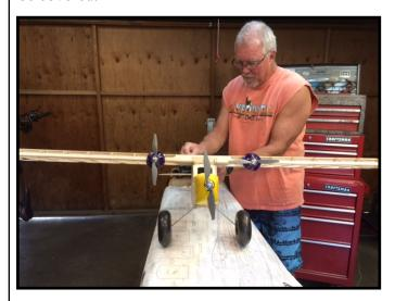
This plane is based on the Great Planes Electric Cub kit, circa 2000. The nearly complete tri-plane wing is being assembled by the handsome owner. Without the front motor, the battery would have to protrude out the front of the cowl to achieve the correct center of gravity Note the tundra wheels - another engineering change implemented due to the owner's apparent lack of ability to land on the infield. This is a relatively large plane for a park flyer, with a 59-in wingspan.
