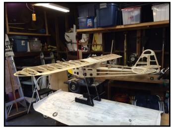
Just to prove the plane really does balance correctly, this is a shot of it on the balancer, ready for covering.
