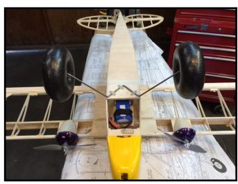
The bottom of the plane allows access to the battery and hatch cover. The 3S-2200ma battery is still in front of the CG by several cm, which allows easy adjustment of the CG.
